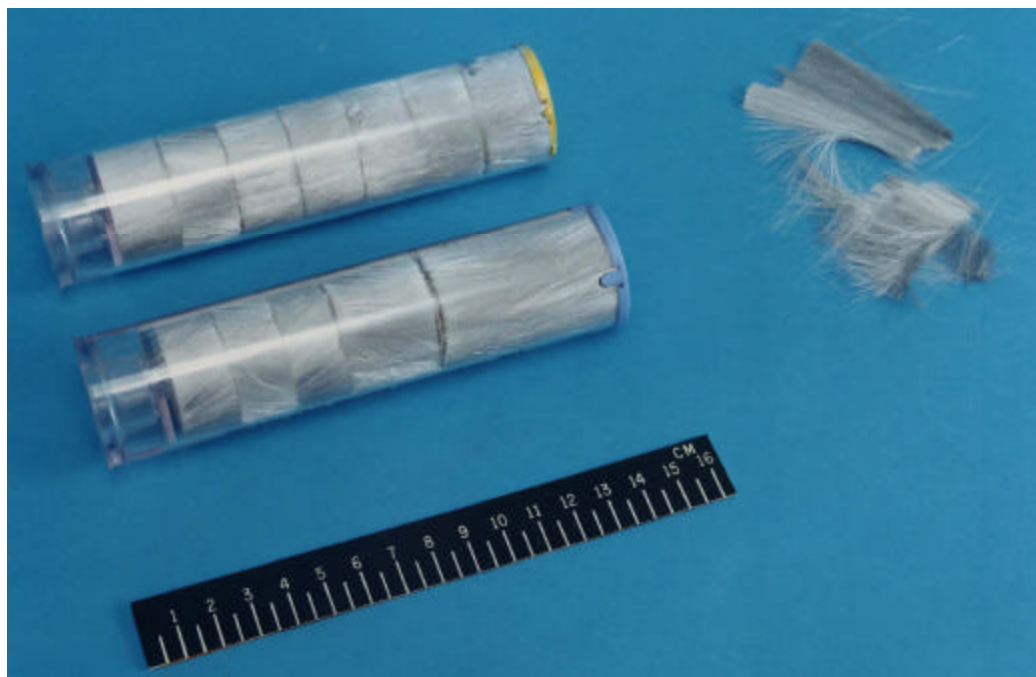
Training and operation RF chaff rounds used by the USN. RR-144 (top) and RR-129 (bottom).
